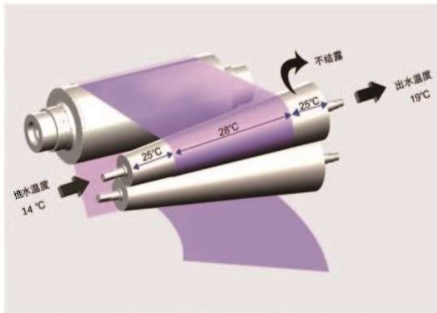
無結露冷卻滾筒-----不結露 Non-condensing cooling roller : not easy to condense
